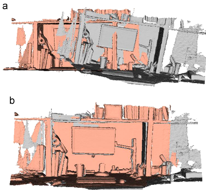
Fig. 16. Registration results of the desk obtained via Kinect. (a) Shows the two raw models obtained from a different views. (b) Shows the registration result.
